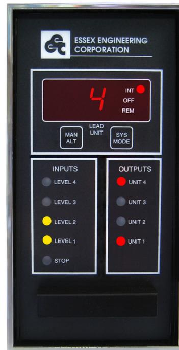
manual pushbutton on the instrument face. When in the REMOTE mode, the unit can be alternated by the use of an external device such as a time clock, pushbutton, etc..
