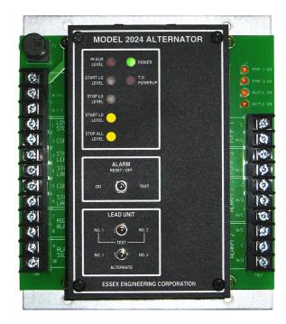
High level alarm point can be field set for lock-in, manual reset, or automatic reset. Relay K4 can follow K3 for DPDT switch operation, or be used as an audible device relay, dropping out when Alarm Silence pushbutton is added.
