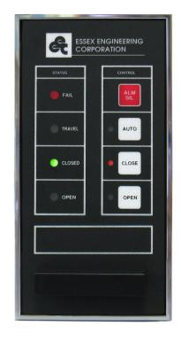
A time delay valve failure monitoring system is standard equipment, and is field adjustable from 0.2 to 60 seconds. If the valve does not operate within the specified time, the red FAIL indicating light will come on steadily. When coupled with the Essex Model 2401 Alarm Module, the red FAIL indicator on the 2403 will flash and an audible alarm will sound from the 2401. By pushing the alarm button on either the 2401 or 2403, the alarm will be silenced, and the red FAIL light will glow steady.
