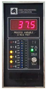
Fill/empty action is field selectable for each control point via the setpoints. Three alarms, each of which has an LED indicator, are provided. These are high and low level, with a signal loss causing the red signal loss LED to flash when activated. The 2410 Controller may be field programmed, via internal DIP switches, to deenergize the control outputs when any alarm condition occurs. An external input signal is also available to deactivate the control and/or alarms when activated.
